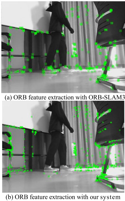
Fig. 14. Comparison of ORB-SLAM3 with ORB feature extraction in our system. This method removes the dynamic features of the walking human body.
