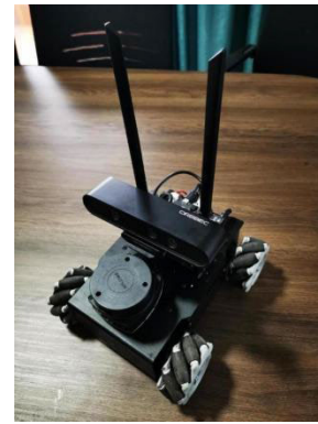
Fig. 12. Mobile robot and Astra Pro camera.
