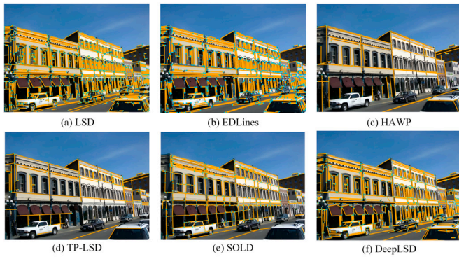
Fig. 6. The comparison of line feature detection methods: Performance of traditional methods and deep learning methods on the YorkUrban dataset. (Akinlar & Topal, 2011; Huang et al., 2020; Pautrat and Barath et al., 2023; Pautrat, Lin, Larsson, Oswald, & Pollefeys, 2021; Von Gioi et al., 2008; Xue et al., 2023)
