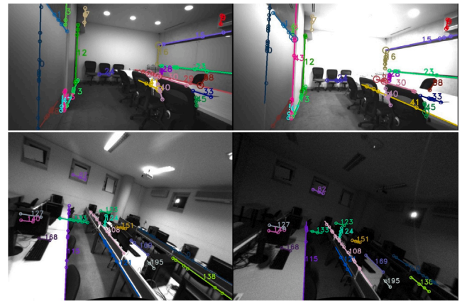
Fig. 13. Line Matching in Challenging Scenes by Xu et al. (2023). The matched lines are depicted in the same color. Circles on the lines represent points associated with each line.
